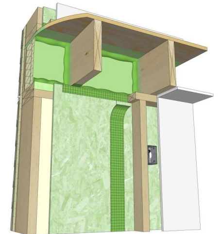
Sealed Sheathing (with service cavity)
