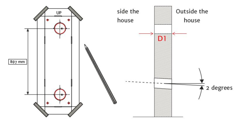
STEP 1: Choose the place Use drilling template Mark the holes
