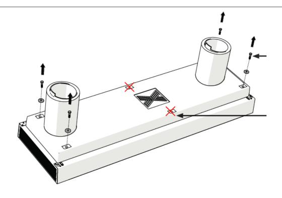
STEP 4: Glue the lower pipe Push fit the upper pipe Fit the insulation tube Remove the 4 bolts
