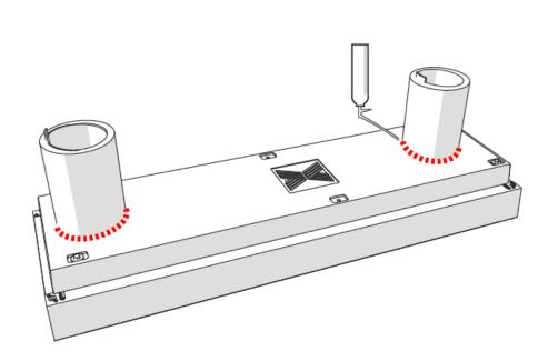
STEP 5: Seal off with PUR Install the unit onto the wall
