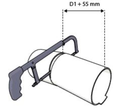
STEP 3: Cut the pipes to length
